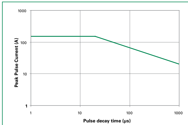
Figure 1: Non-repetitive Peak Pulse Current vs. Pulse Time
