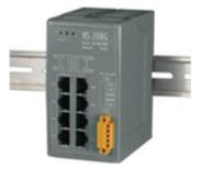
The NS-208G has 8 Ethernet Switching ports that support 10/100/1000 Base-T, with a 10/100/1000M auto-negotiation feature and auto MDI/MDIX function. It can connect 8 workstations and automatically switches the transmission speed (10 Mbps or 100 Mbps or 1000Mbps) for corresponding connections. The flow control mechanism is also negotiated. There is link/data rate LEDs for each port to aid trouble-shooting. Port connectors are shielded RJ-45.
