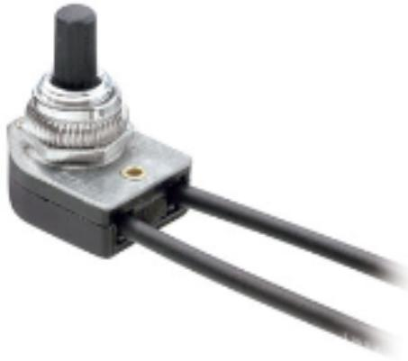
Rotary switch, single pole on-off; 6A-125VAC, 3A-250VAC; male bushing 3/8-27 by 11/32 inch long thread. Two 6 inch black leads 18AWG AWM TEW 105C 600 V plastic, free ends stripped 1/2 inch.
