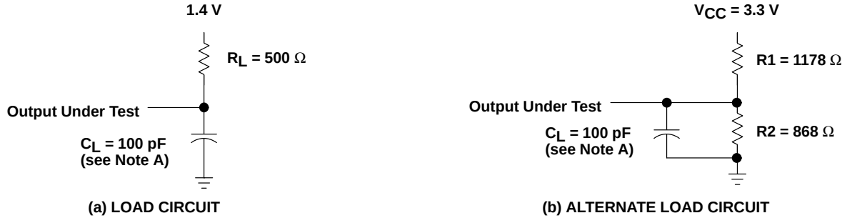
Figure 3. Low-Voltage Load Circuits for Timing Parameters
