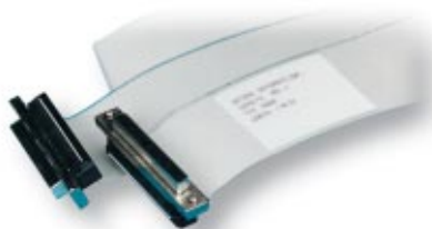
Figure 10. R6868 Ribbon I/O Cable
