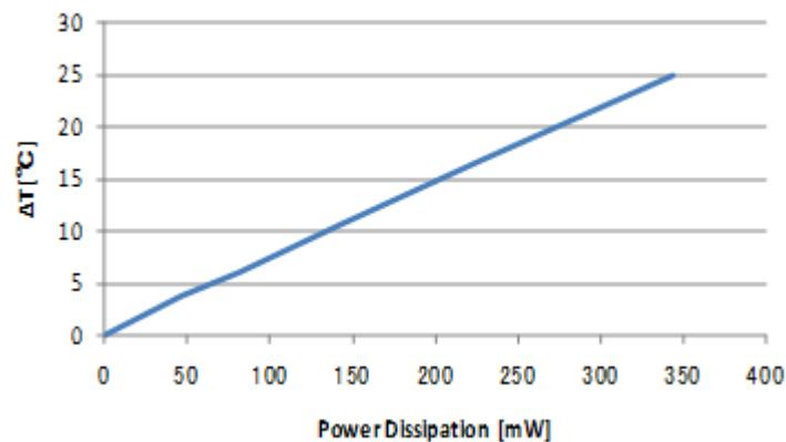
The output current of the device may need to be de-rated if it is operated in high ambient temperature or in an application that requires continuous power delivery. The amount of current de-rating is highly dependent on the environmental thermal conditions, e.g., PCB design, nearby components, or effective air flow. Care should especially be taken in applications where the device temperature exceeds 85°C.
