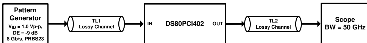
Figure 9-2. Test Setup Connections Diagram
