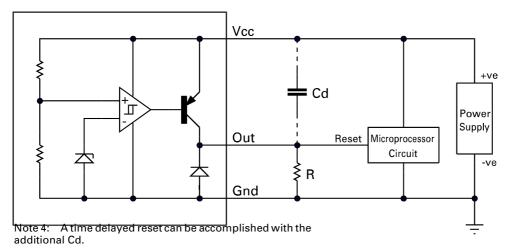
$$T_{DY} = RCd \left[ ln \left( \frac{1}{V_{TH}} \right) - ln \left( \frac{1}{1 - \frac{V_{SAT}}{V_{in}}} \right) \right]$$
