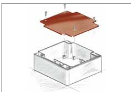
Standard mounting bosses, in some cases also fitted in the lid.
