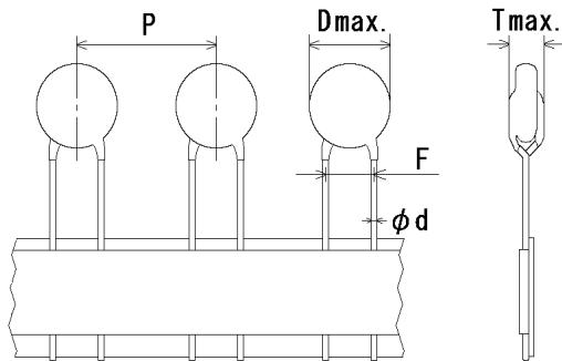
Note) The mark '\*' of lead code differ from lead spacing(F), lead diameter(d) and pitch of component(P).
