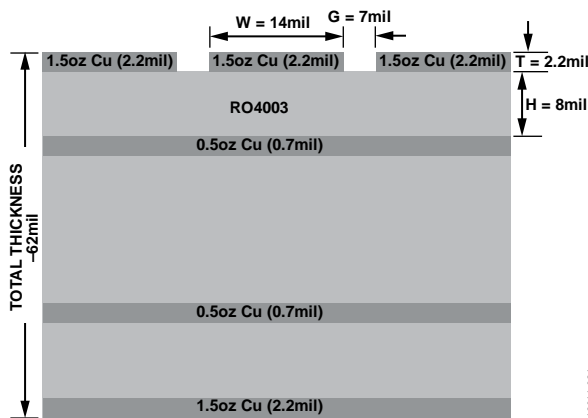
Figure 22. Probe Matrix Board (Cross Section View)
