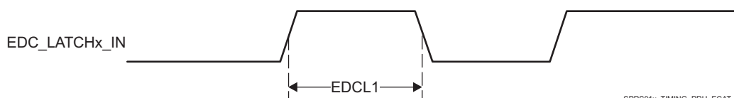
Figure 5-120. PRU-ICSS ECAT LATCHx_IN Timing
