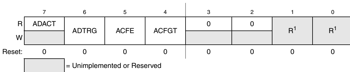
Figure 8-5. Status and Control Register 2 (ADCSC2)
