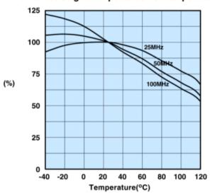
Measured on a 2643000301 using the HP4291A.
