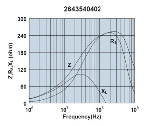
Impedance, reactance, and resistance vs. frequency.
