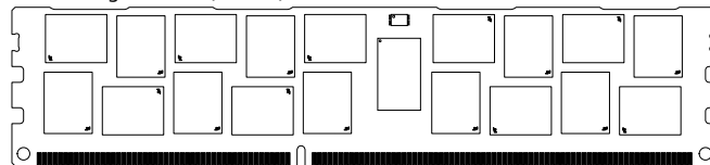
Figure 1: 240-Pin RDIMM (R/C E2)
