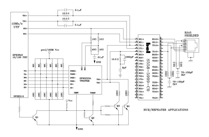
**NOTE:** It is recommended for the above application to leave the secondary side center taps unconnected. For applications with other IC's, please consult the factory for recommendations on center tap termination and layout schematic.
