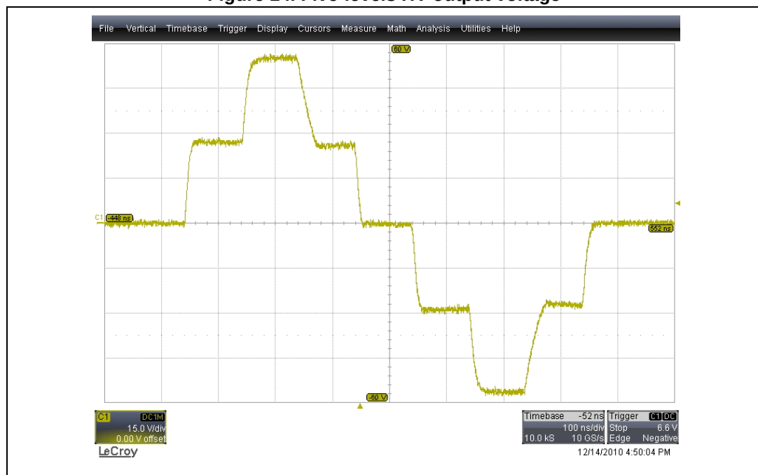
Figure 14. Five-levels HV output voltage
