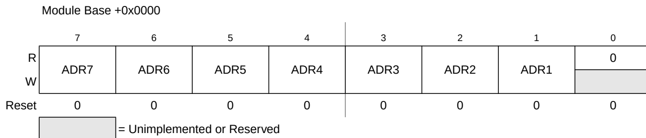
Figure 10-3. IIC Bus Address Register (IBAD)
