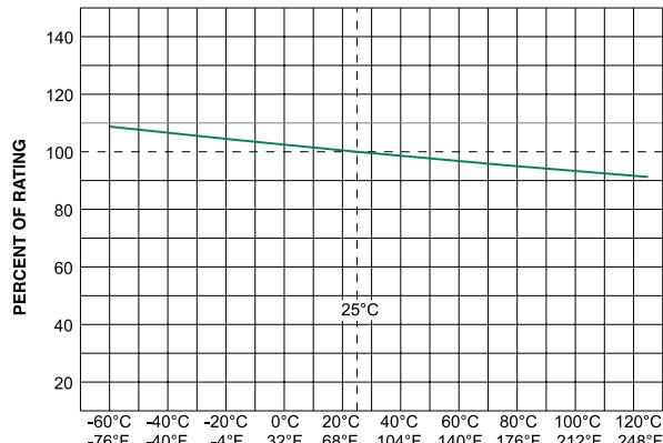
**NOTE:** Derating depicted in this curve is in addition to the standard derating of 25% for continuous operation.
