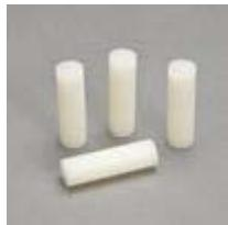
A high performance hot melt adhesive for bonding many plastics including polyethylene and polypropylene. It has excellent thermal shock, good heat resistance, good electrical properties, and it is non-corrosive to copper. Designed for use through 3M™ Scotch-Weld™ Hot Melt Applicator, TC.
