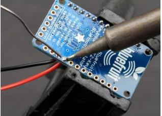
Strip the wires and solder them to the Vin and Gnd holes.
