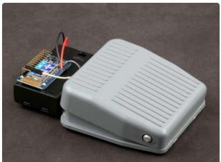
Connect the jumper to pin #1 of the rightangle header. And you are ready to go!
