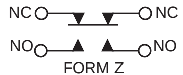
Circuit for microswitch version
