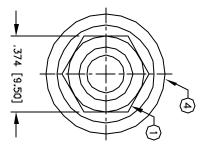
SCREW CONNECTOR ONTO CABLE IN A CLOCKWISE DIRECTION UNTIL IT STOPS
