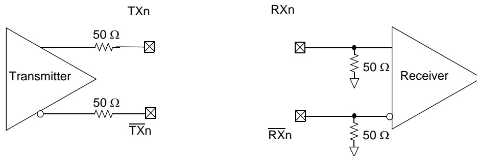
Figure 48. SerDes Transmitter and Receiver Reference Circuits
