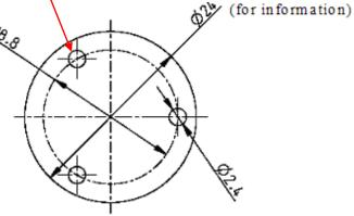
Dimensions tolerance is +/-0.2mm
