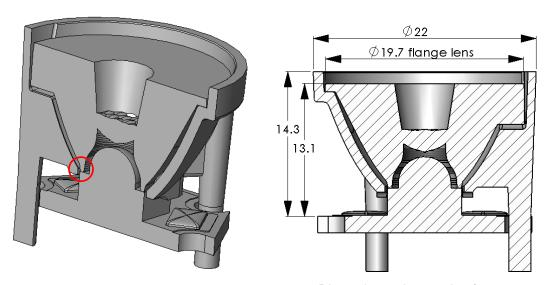
Dimensions tolerance is +/-0.2mm
