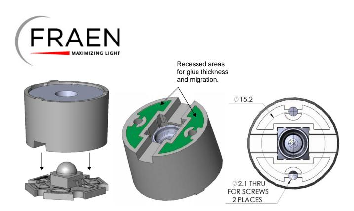
The lens assembly can be secured to the PC board by using glue or silicone RTV. To avoid glue on the lens and LED, apply it along the outside diameter edge, or apply a very thin film on areas shown above in green. Alternatively, screws can be used for example ISO1481-ST2.9 metric.
