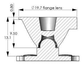
Dimensions of lens on K2 LED (lens shown without lens holder):
