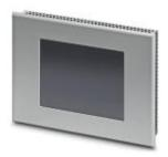
Touch panel with 38.1 cm/15" TFT-display (Resistive industrial touch screen), 1024 x 768 pixel(s) (XGA), 65536 colors, Xscale® PXA320, 806 MHz, 2x USB Host 1.1, 1x Compact Flash®, 1 x Ethernet (10/100 Mbps), RJ45, Windows CE 5.0 and user software: Visu+ / AX OPC Server. (bus system: without)
