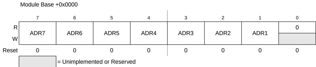
Figure 10-3. IIC Bus Address Register (IBAD)
