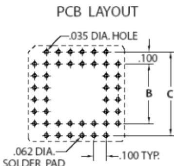
FOR PRINTED CIRCUIT DRILLING PATTERNS
