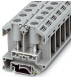
Universal terminal block with bolt connection, cross section: 1 - 25 mm 2 , width: 18 mm, color: gray
