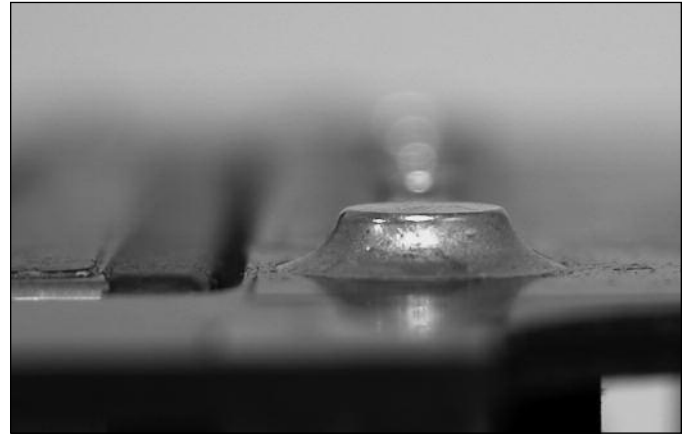
Figure 23–1 — Side profile of a Mini module solder joint
