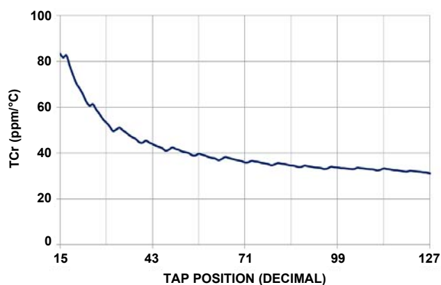
FIGURE 16. 50kΩ TCr vs TAP POSITION, V_{CC} = 3.3V
