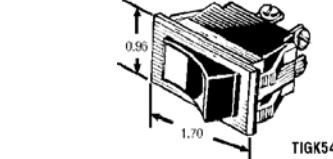
These full-size rocker switches are designed for AC and low voltage DC applications. They include a slow make, slow break contact mechanism, nylon snap-in brackets and are available to resolve most insulation requirements. They are rated at 15 amps 125 VAC, 28 VDC, 10 amps 250 VAC 3/4 H.P. UL recognized and CSA certified.
