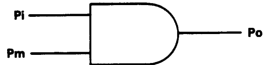
Figure 5. Equivalent Logical Representation of Masking Operation
