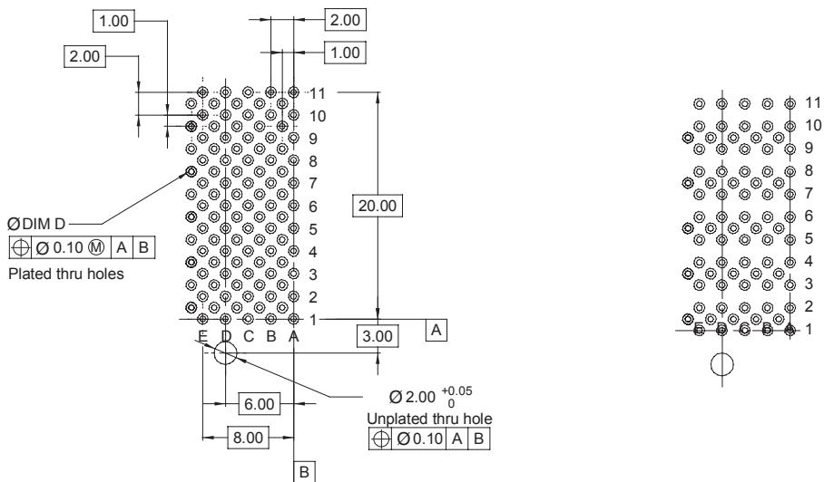
Recommended PCB hole mounting pattern for coaxial,
