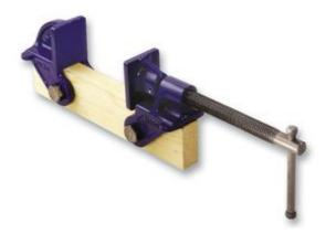
Clamp Heads are an economical alternative to the full size bar clamps. The Head and Slide with steel mainscrew can be fitted to a wooden batten 25 mm (1") thick by 38 mm (1  $\frac{1}{2}$ ") wide, and of any desired length. The timber is then drilled with two 11.1mm (6/16") diameter holes producing a light duty bar clamp as strong and true as the timber you choose.
