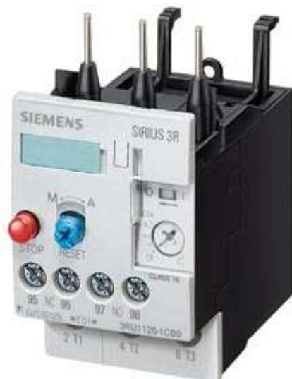
OVERLOAD RELAY,11...16 A, 1NO+1NC, SIZE S0, CLASS 10, FOR CONTACTOR MOUNTING
