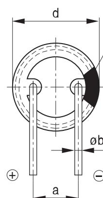
The series B41898 has no sleeve nor minus pole marking, the positive pole is marked on the aluminum case side instead.
