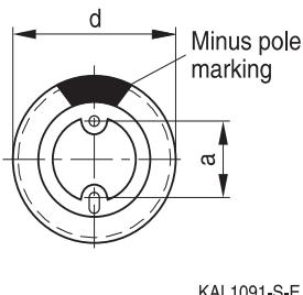
The series B41898 has no sleeve nor minus pole marking, the positive pole is marked on the aluminum case side instead.
