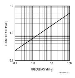
Figure 11. Attenuation vs Frequency for Belden 9481
