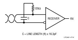
Figure 14. AC Coupled Termination
