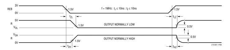
Figure 8. Receiver Enable and Disable Times
