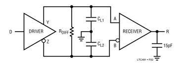
Figure 2. Driver/Receiver Timing Test Circuit
