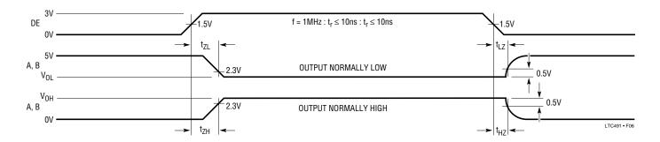
Figure 6. Driver Enable and Disable Times
