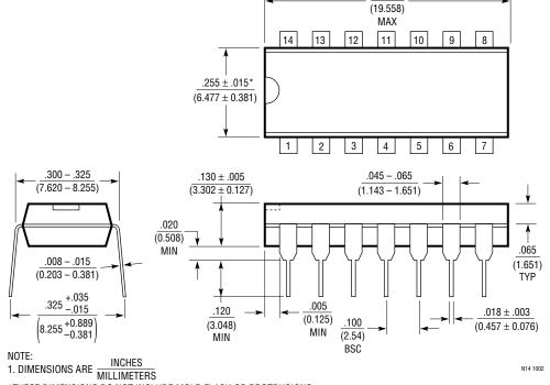
\*THESE DIMENSIONS DO NOT INCLUDE MOLD FLASH OR PROTRUSIONS. MOLD FLASH OR PROTRUSIONS SHALL NOT EXCEED .010 INCH (0.254mm)
