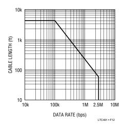
Figure 12. Cable Length vs Data Rate
