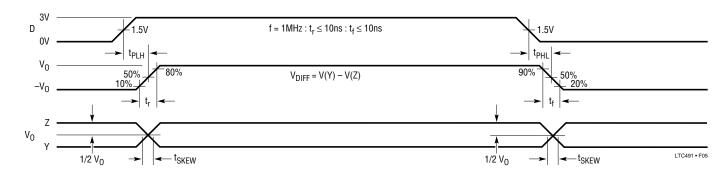
Figure 5. Driver Propagation Delays
