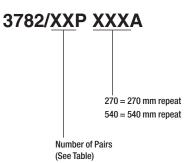
Note: Available in standard 100 ft rolls. Contact 3M for availability of additional conductor counts and/or custom roll lengths.
