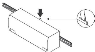
Press button downwards (to unlock) and remove the unit from the DIN Rail.
