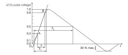
Front time:  $T_1 = 1.67 \text{ x T} = 1.2 \text{ } \mu \text{s} \pm 30 \text{ } \%$
