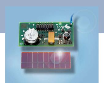
The STM 110 module serves the 868 MHz air interface protocol of EnOcean. Together with the receiver modules RCM120 and RCM 130 this module can be easily implemented into operation and control units for realization of various application specific system solutions.
