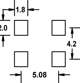
Dimensions are in millimeters.
