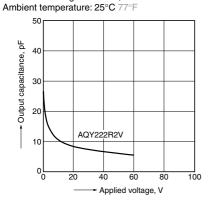
12.-(2) Output capacitance vs. applied voltage characteristics
