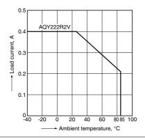
1.-(2) Load current vs. ambient temperature characteristics
