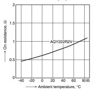
2.-(2) On resistance vs. ambient temperature characteristics
