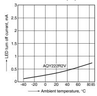
6.-(2) LED turn off current vs. ambient temperature characteristics Load voltage: 10V (DC); Continuous load current: 80mA (DC)
