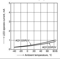
6.-(1) LED turn off current vs. ambient temperature characteristics Load voltage: 10V (DC);
