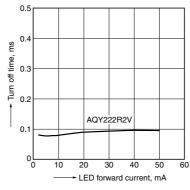
11.-(2) Turn off time vs. LED forward current
