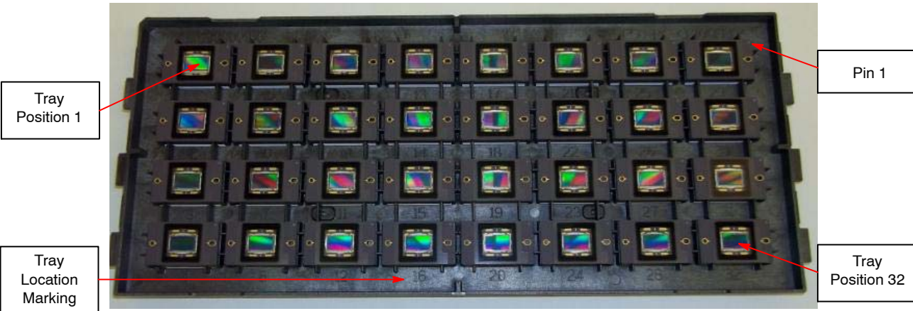
Figure 35. Tray Pin-Down View
