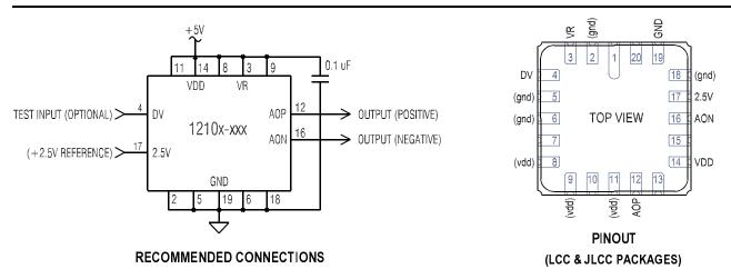
The 2.5V reference input may be driven from either a precision voltage source or a  $5k\Omega/5k\Omega$  resistive divider from a precision 5V supply. If a resistive divider is used, a 0.01µF bypass capacitor should be connected between the 2.5V input and GND.
