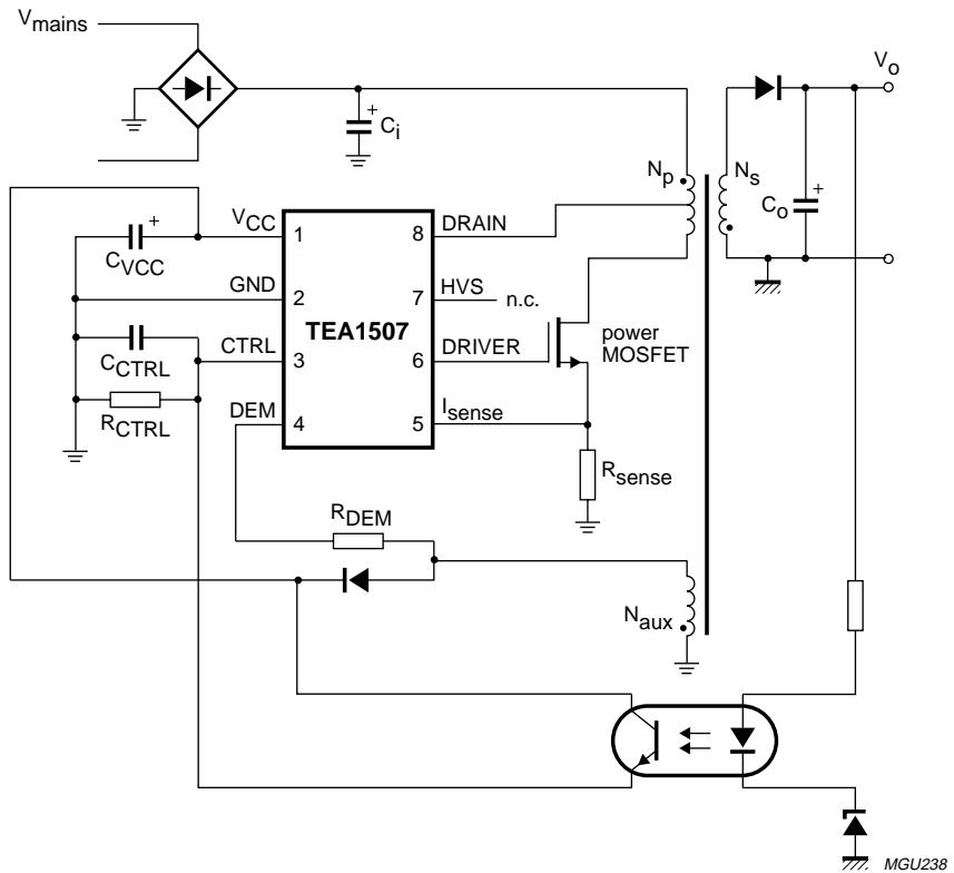
Fig.10 Flyback configuration with secondary sensing.
