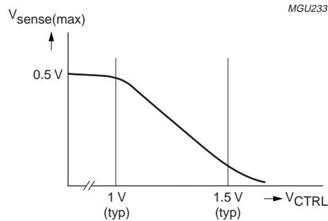
Fig.5 The  $V_{sense(max)}$  voltage as function of  $V_{CTRL}$ .
