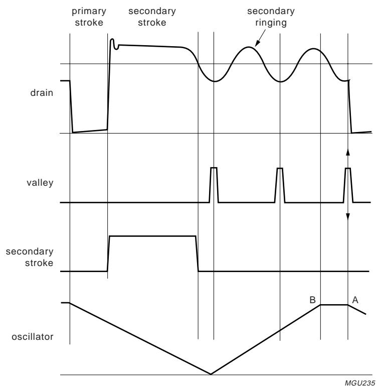
A: Start of new cycle at lowest drain voltage.
