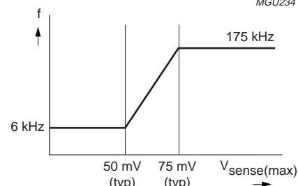
Fig.6 The VCO frequency as function of  $V_{sense(max)}$
