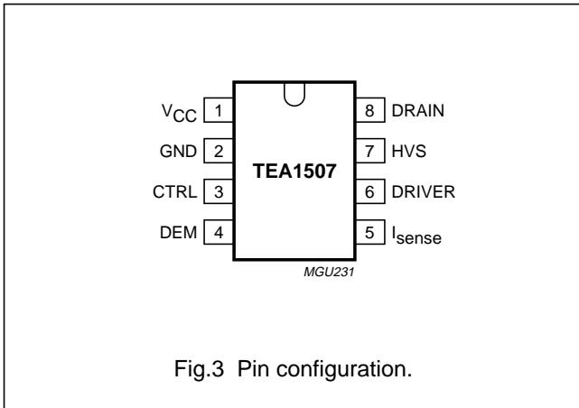
Fig.3 Pin configuration.
