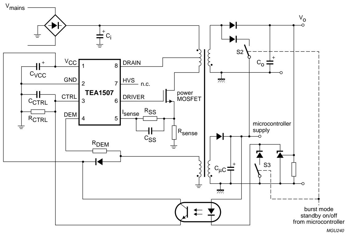
Fig.12 Flyback configuration with secondary sensing using the burst mode standby.
