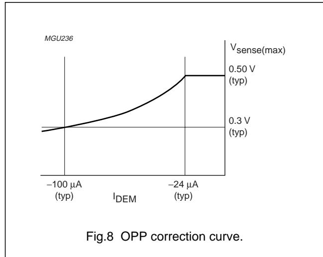
Fig.8 OPP correction curve.
