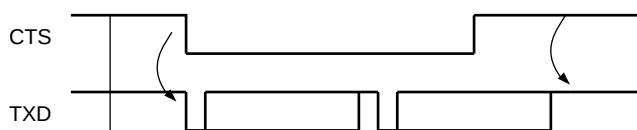
Figure 31-21. Transmitter Behavior when Operating with Hardware Handshaking
