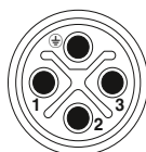
Pin assignment of M12 plug, 4-pos., S-coded, view of plug side
