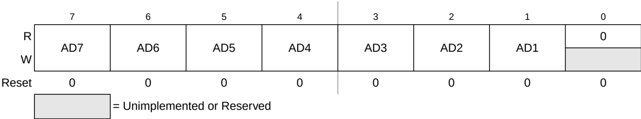
Figure 11-3. IIC Address Register (IICA)
